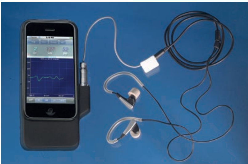
PulsEar - the earphone that measures your heart rate © CSEM
