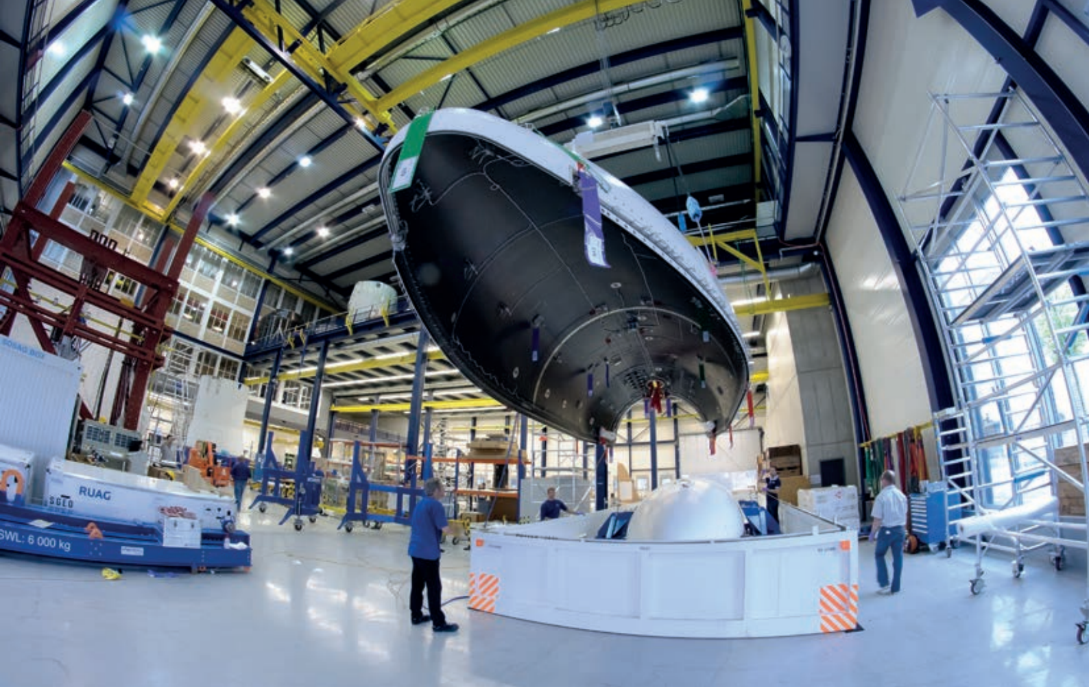
The payload fairing for a Vega rocket is packed for transportation at RUAG Space in Zurich © RUAG
