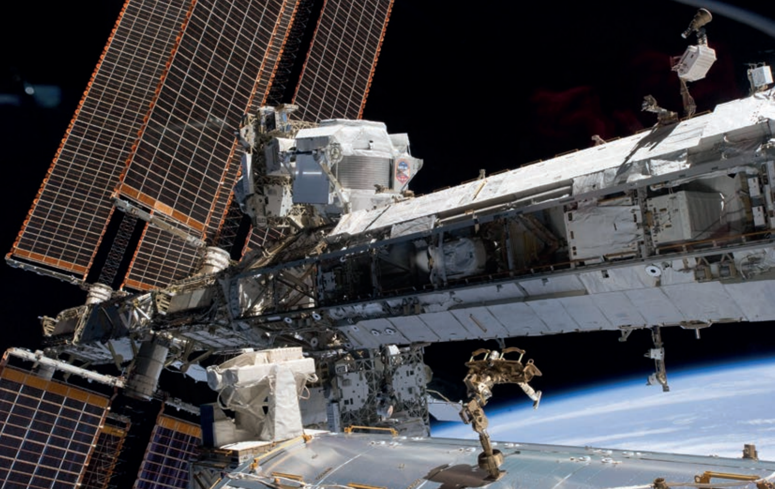
The Alpha Magnetic Spectrometer, installed on the truss section of the International Space Station © NASA
