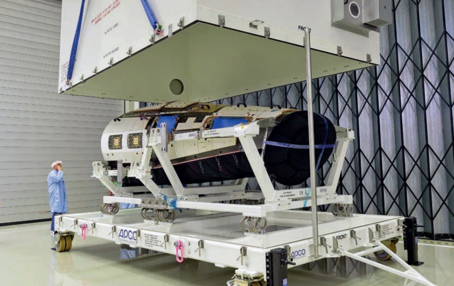
Structure of the European Intermediate eXperimental Vehicle IXV, built by RUAG Space, handled by APCO Technologies' Mechanical Ground Support Equipment © ESA
